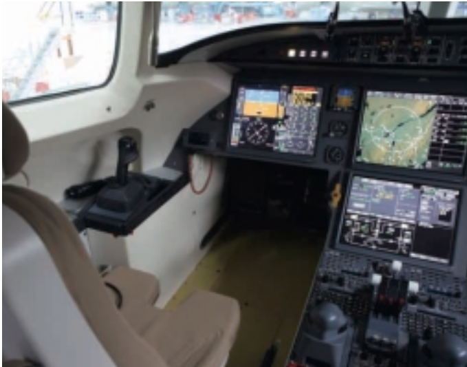
Advanced cockpit technologies incorporated into Dassault's EASy flight deck (left) are designed to make piloting new business jets more intuitive. The 13-passenger Embraer Legacy (right) is the largest and newest aircraft offered by fractional provider Flight Options.
